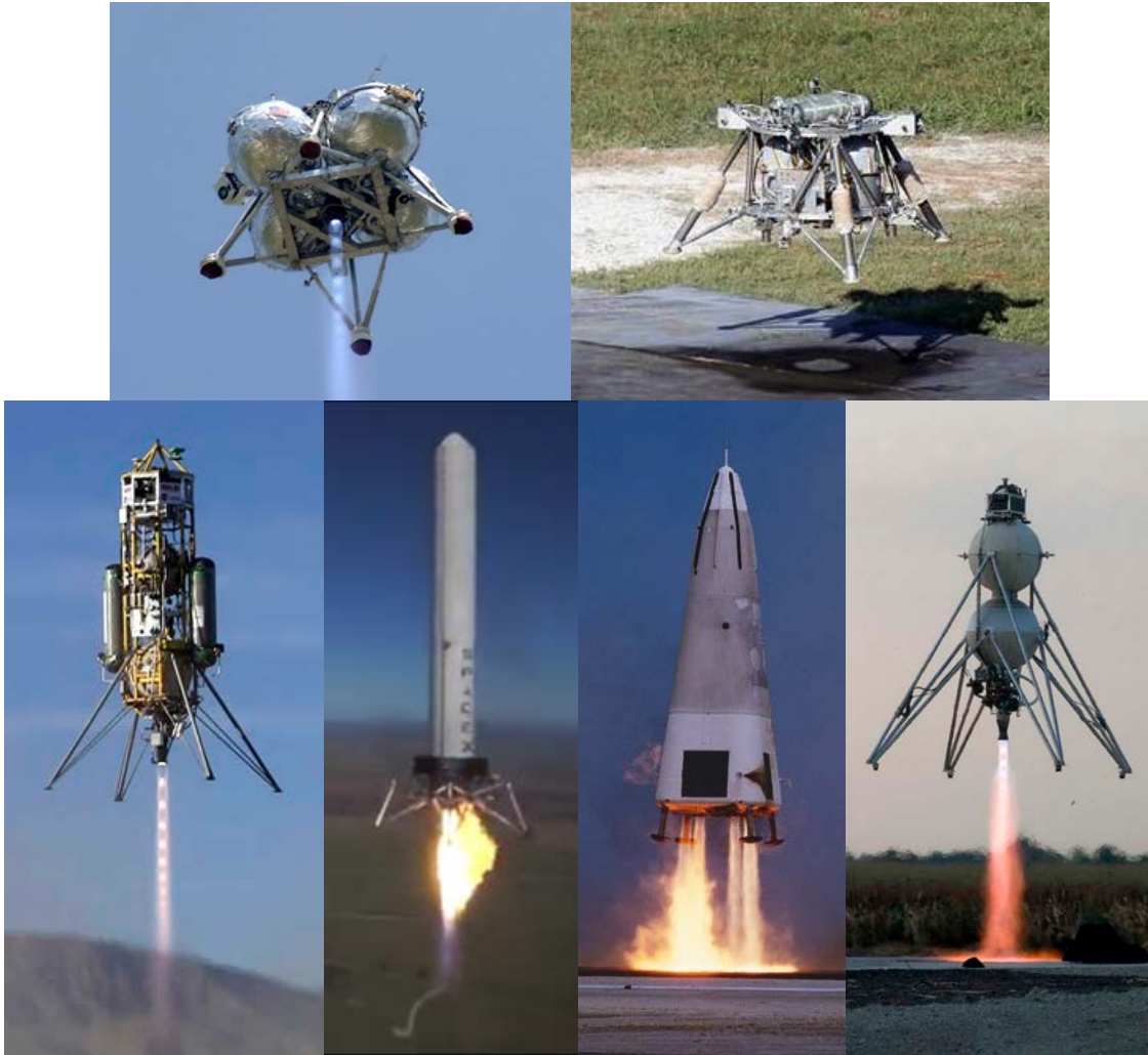
Figure 6: Various experimental Vertical Takeoff and Landing testbeds. Clockwise from top left: Morpheus, Mighty Eagle, Xombie, Grasshopper, DC-X and Mod
